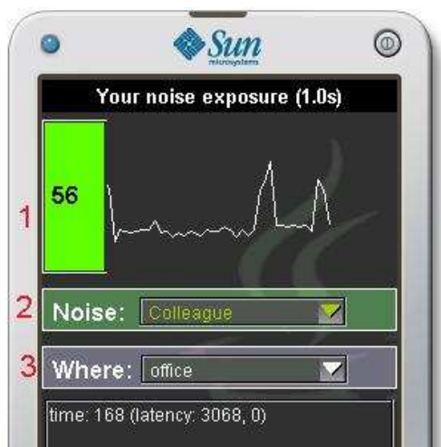
Figure 2. The Mobile sensing application. Including 3 components: (1) The visualization of the loudness measured and a color representing the danger (2) The noise tagging (3) The tagging of the location (for indoor location for instance)
